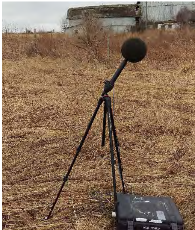
Figure 1-9 Location 3 – Winter Sound Level Meter
