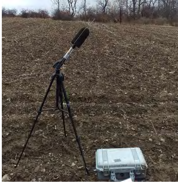
Figure 1-5 Location 2 - Winter, Sound Level Meter
