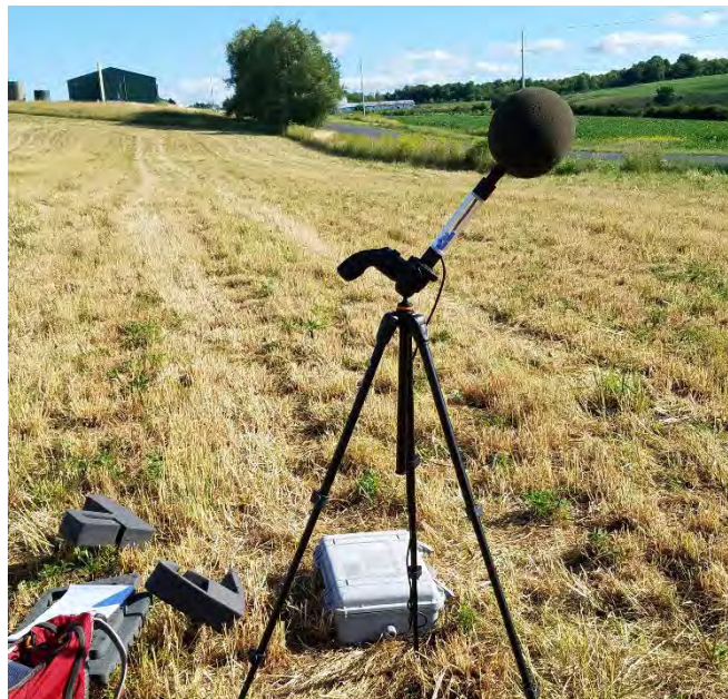
Figure 1-4 Location 2 - Summer, Sound Level Meter
